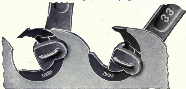
Method of Using Chisel Tooth Wrench
