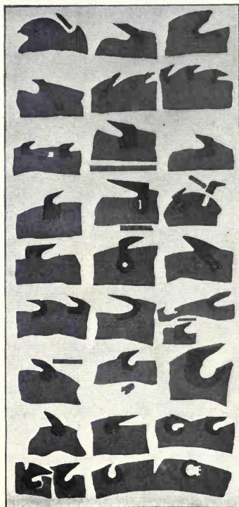
Early Types of Inserted Teeth for Circular Saws
